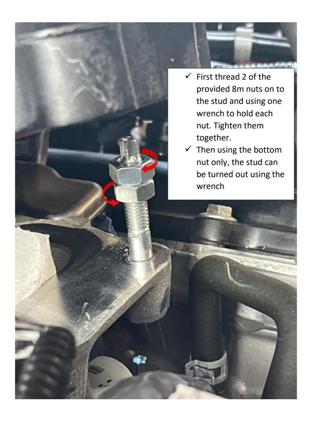
8. Once the 2 studs are removed. Also remove the paper towels or cloth from the intake ports and ensure the original gasket is still in place.
