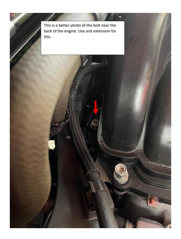
7. Lift the Intake Plenum off the lower intake and set off to the side. If doing this alone, use bungee ties to hold the intake up as your working under the hood. The 2 Studs will need to be removed.
