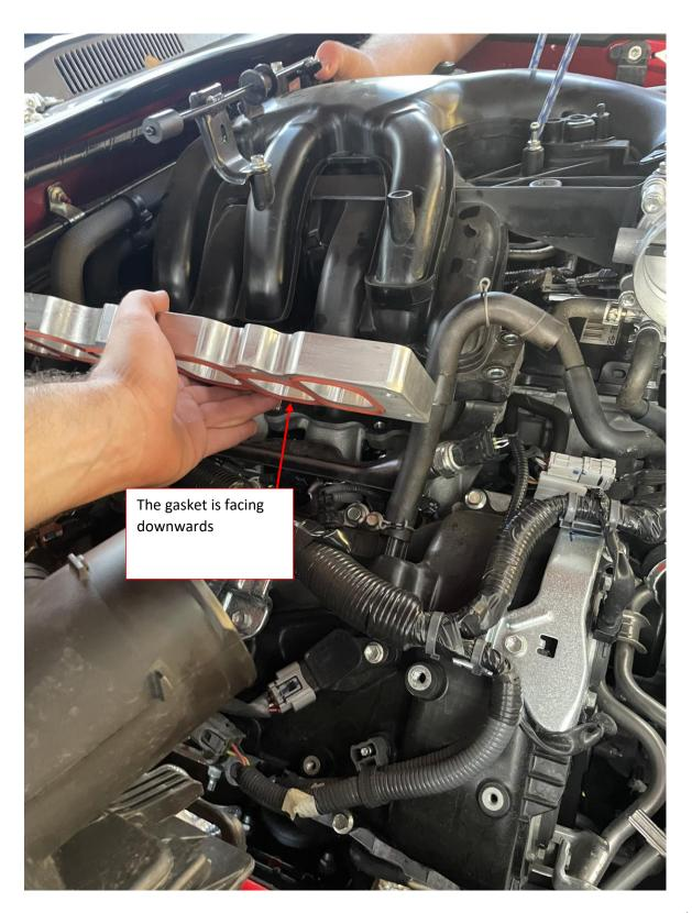
10. Using the provided Bolts 8 total (8m x 1.25 (65mm long)), positions the intake space to align all the bolt holes. Use one Lock washer and round washer on each bolt and torque to 10 - 12 ft.lbs
