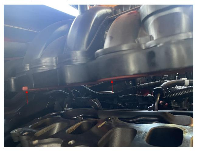
9. Place the intake manifold Spacer between the upper and lower intake ensuring the gaskets is facing down. The spacer will only go in one way.
