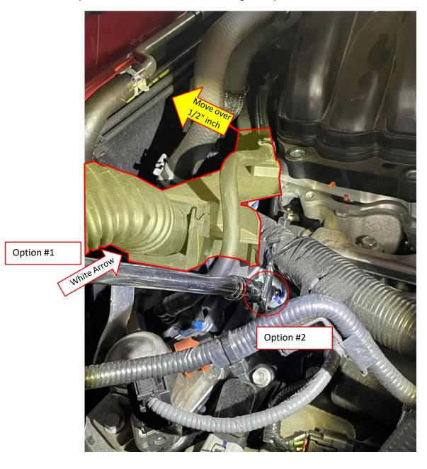
6. Unbolt the 8 total positions on tops the intake holding the plenum on. Depending on model, year, and trim level. There may be one unused bolt positions therefore you'll only need to unbolt 7 bolts.
