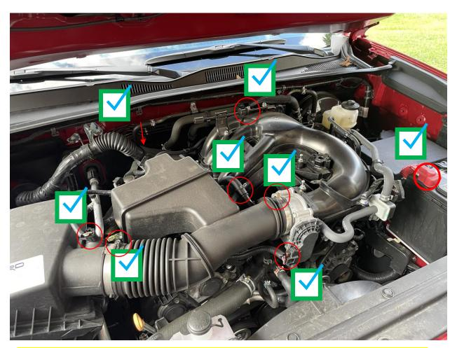
Ensure the 3 Small brackets are used at the manifold support locations, there are 2 on the driver-side of the manifold and 1 location on the front.
