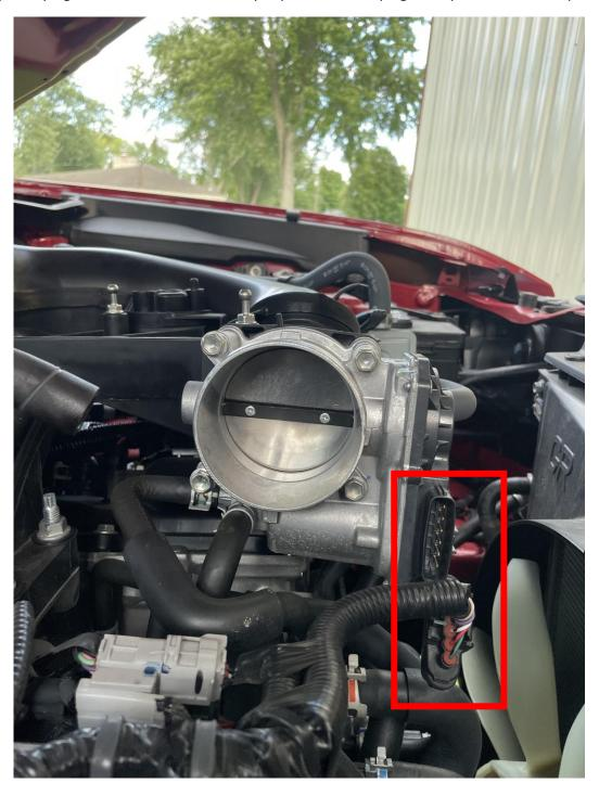
5. The Wiring harness bracket will need to be unclip from the "hanger" at the White Arrow (option 1) **or** you can loosen 2 (10mm) bolts holding the bracket in-place (option 2).
