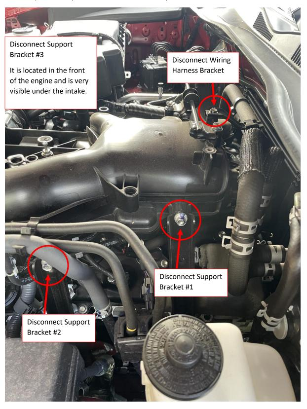
4. Remove the wiring harness clip from the throttle body. The entire throttle body can remain and does not need to be unbolted.
